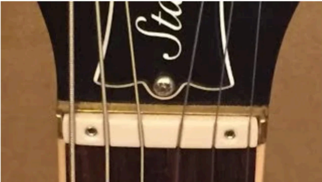
Picture 2. Nut slots filed into an angle. Tune Voodoo not needed.
